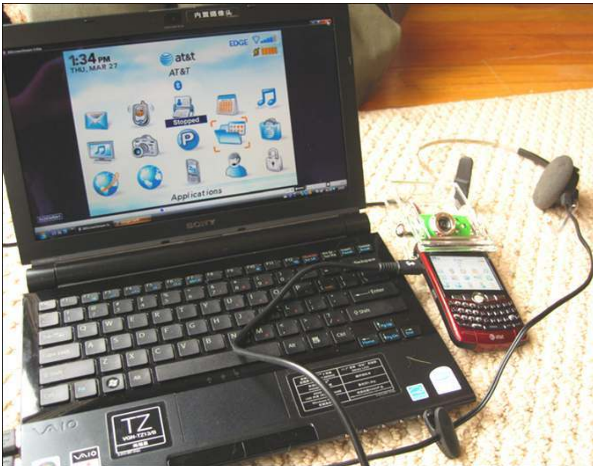
Figure 1: Our equipment set (laptop with built-in camera, BlackBerry with mounted camera, and headset)
